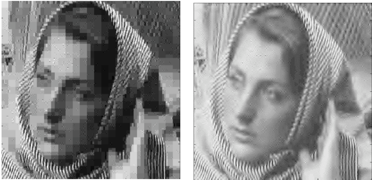
Figure 11.4–5 9 to 1 compression using a set of 2-point Haar filters is shown at left. The same compression using a set of Biorthogonal 7/9 filters is shown at right.
